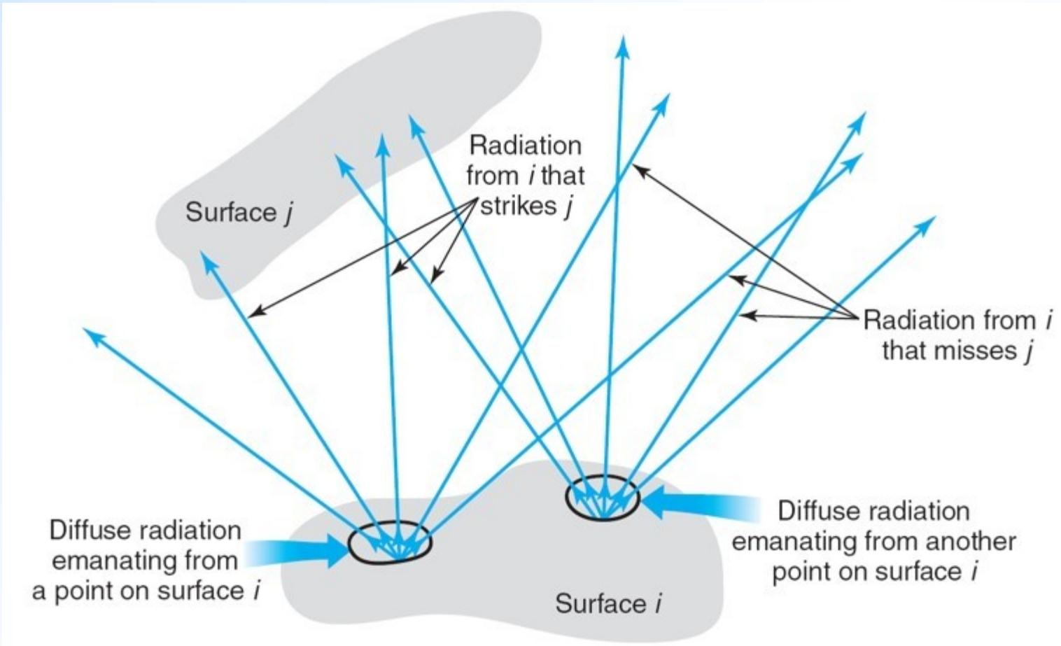
**View Factor:**  $F_{i \rightarrow j}$  is the fraction of diffuse radiation leaving surface *i* that arrives at surface *j* by a straight-line route, and depends on size, orientation and spacing.
