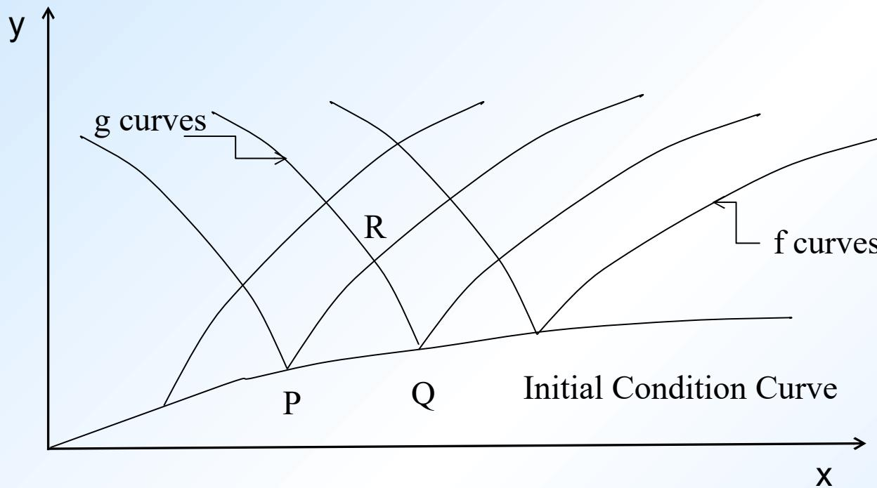
We can obtain a solution at R, by integrating both the characteristic equation and the solution equation from P to R along f curve, and from Q to R along g curve.
