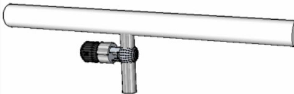
Imagine a device that consists of a pipe with constant radius  $r$  and a valve in which a chemical can be injected. This pipe contains a fluid, for example water.
