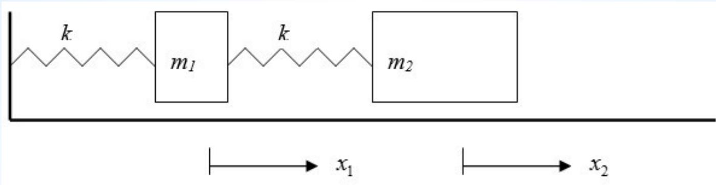
Assume each of the two mass-displacements to be denoted by  $x_1$  and  $x_2$ , both functions of time, and let us assume each spring has the same spring constant,  $k$ .
