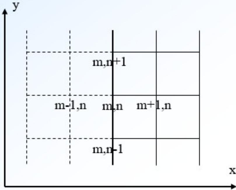
Consider the node  $(m,n)$  on such a boundary. The heat flux in the  $x$ -direction is zero. i.e.,  $q_x = 0$ . Therefore
