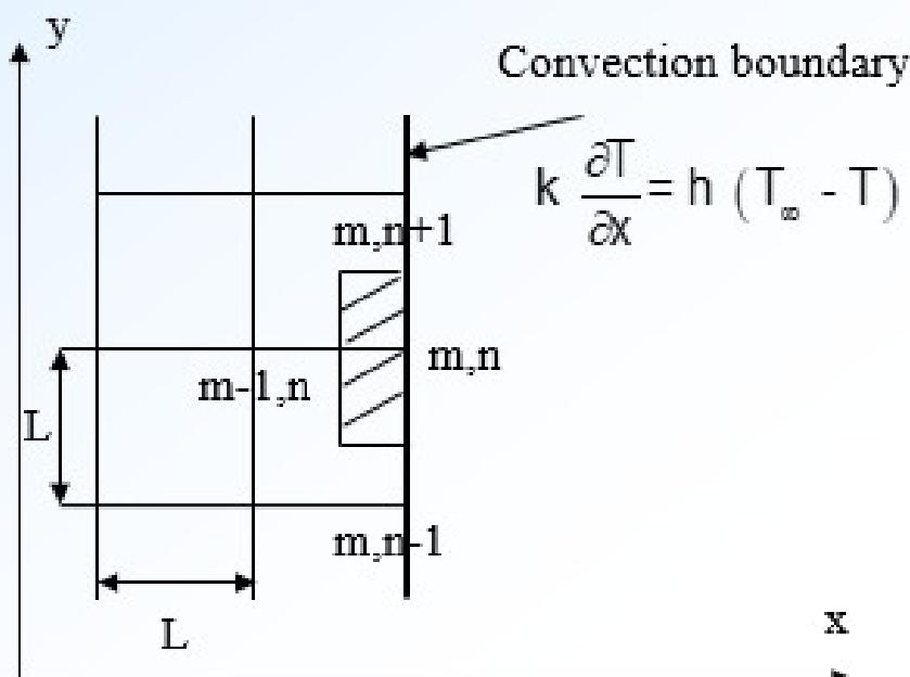
One can find the difference equation for the node  $(m,n)$  by writing an energy balance equation on the shaded volume element (with unit depth).
